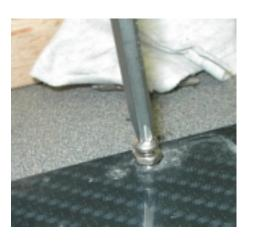
Tighten the fin clamp mounting screws to contact plus an additional ¼ turn.
